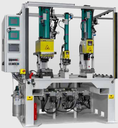
TOX®-Press for eClinching of fuse parts.
